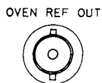
The OVEN REF OUT supplies a 10 \text{ MHz} \pm 1 \times 10^{-7} per month sinusoidal frequency reference from an internal crystal oscillator, located in a temperature-controlled oven. The output is ac coupled and the output impedance is 50 ohms. The nominal output level is +10 dBm/50 ohms. The output is disabled during the oven's warm-up cycle. To use the internal Oven Reference, this output must be connected to the EXT REF IN jack.
