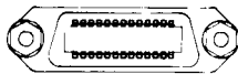
HP-IB Connector: Used to interface the instrument with the Hewlett-Packard Interface Bus (HP-IB) for remote operation. Remote operation is described in the Operating Manual.
